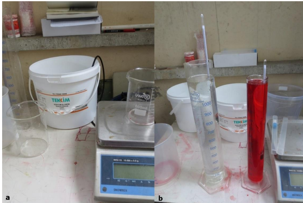
Figure 6.23 : a) Preparation of salt solutions, b) Hydrometers and measurement.
