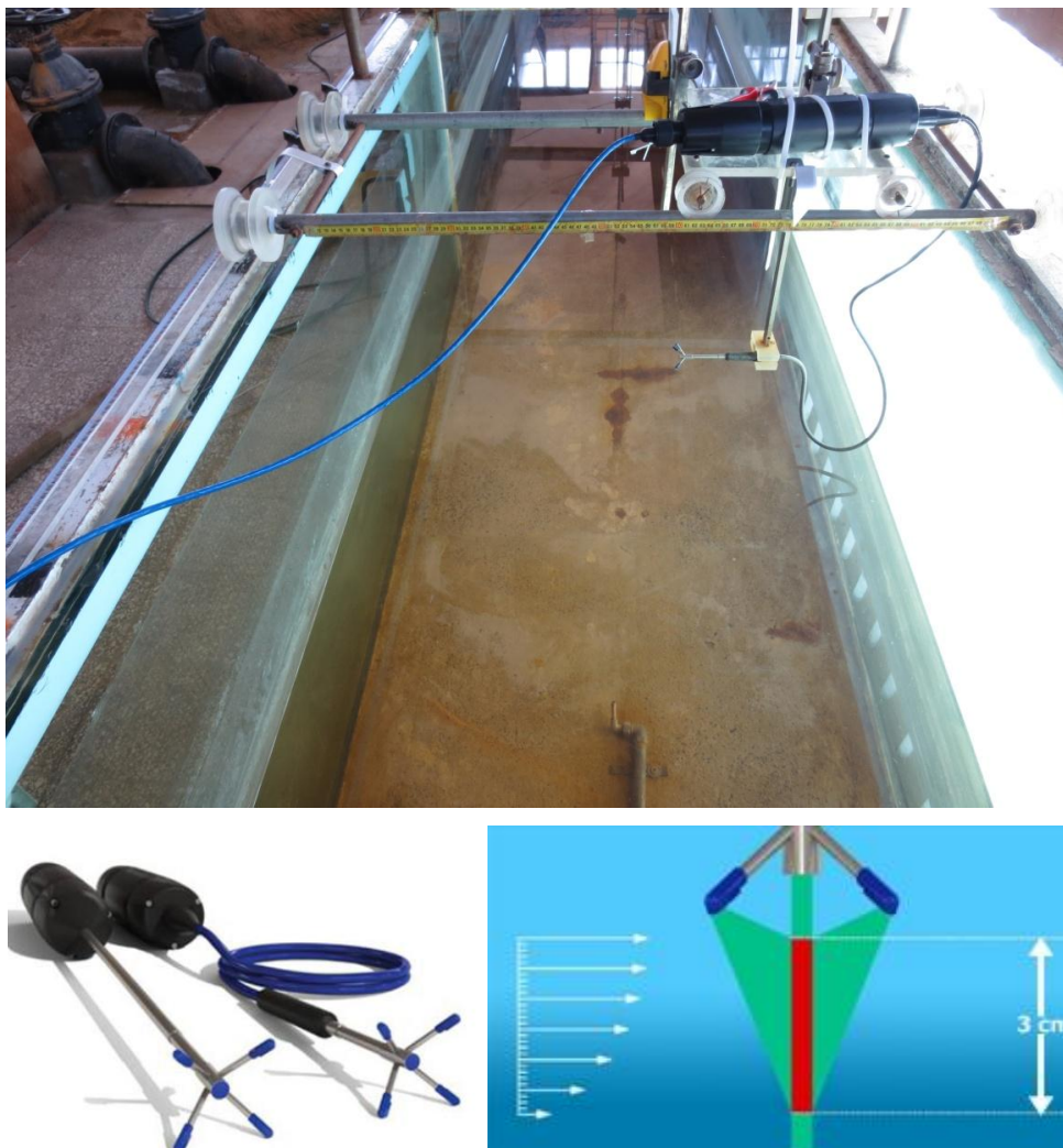
Figure 6.21 : Vectrino II instrument and sampling distance.
