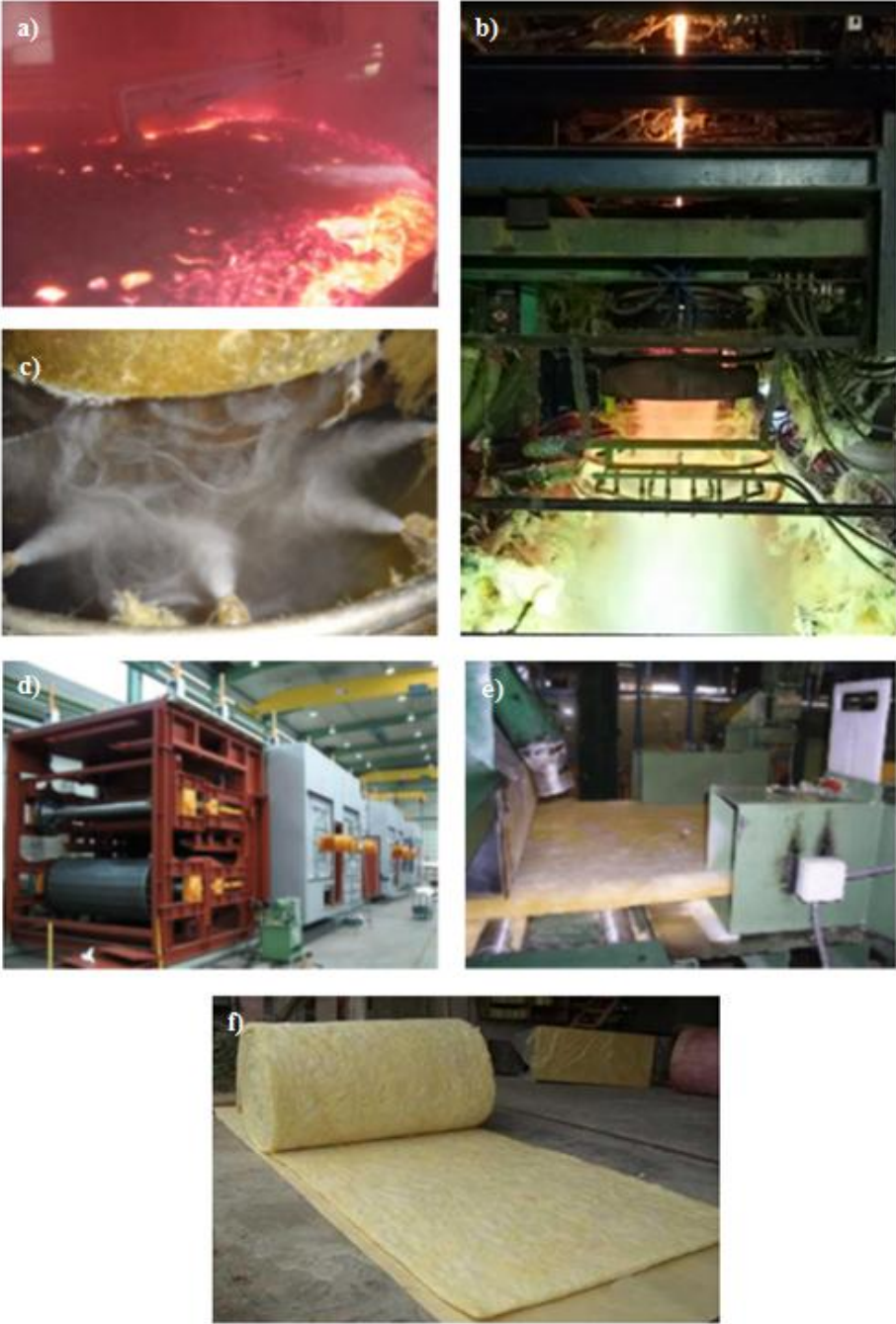
Figure 3.4 : a) The furnace where the raw materials were melted. b) The spinner disc and glass wool. c) Glass wools were sprayed with resol resin samples. d) Curing oven. e) Edge trimmer. f) Composite glass wool insulation product.
