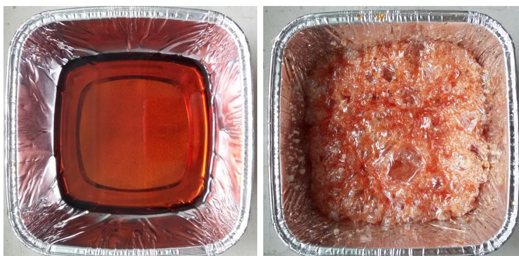
Figure 3.2 : Resol resin (PFR) before drying and after drying process.
