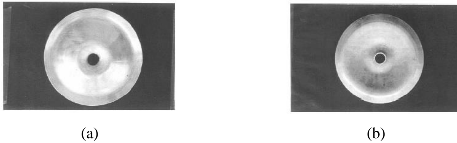
Figure 2.2. Reverse bending (a) top view and (b) bottom view (Source: N. K. Gupta et al., 1997).
