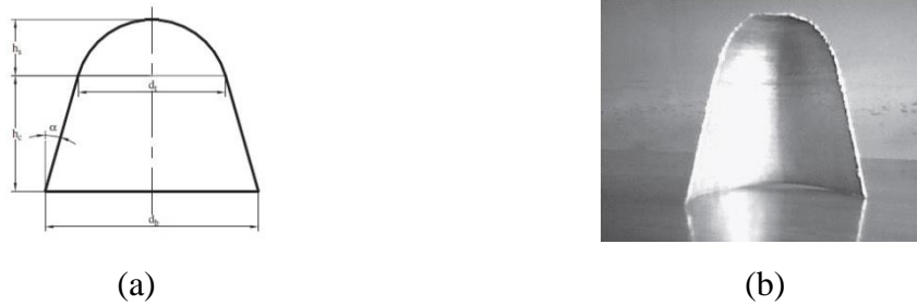
Figure 2.12. (a) Technical drawing of the combined geometry and (b) its sectional view (Source: N. K. Gupta, Mohamed Sheriff, & Velmurugan, 2008).
