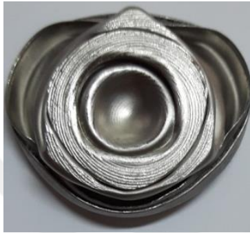
Figure 5.26. Experimentally and numerically crushed specimens at dynamic strain rates; (a) the inner core and (b) balanus structure.
