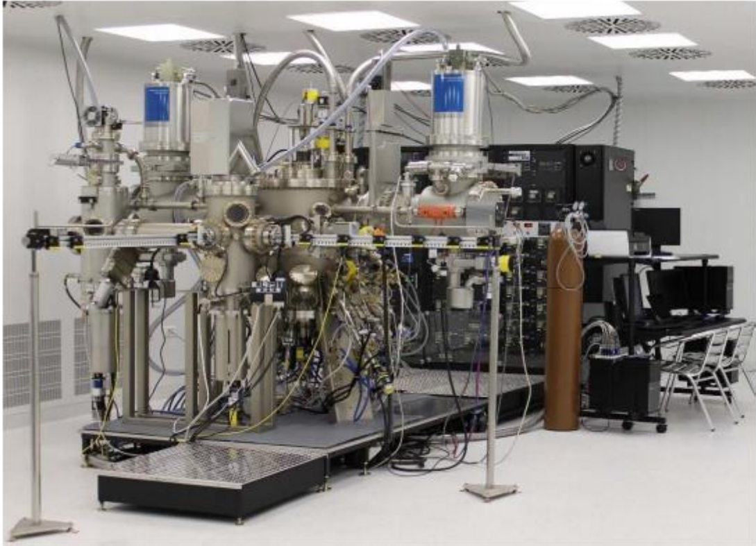
Figure 19. Gen-20MZ MBE system in department of physics in IZTECH
