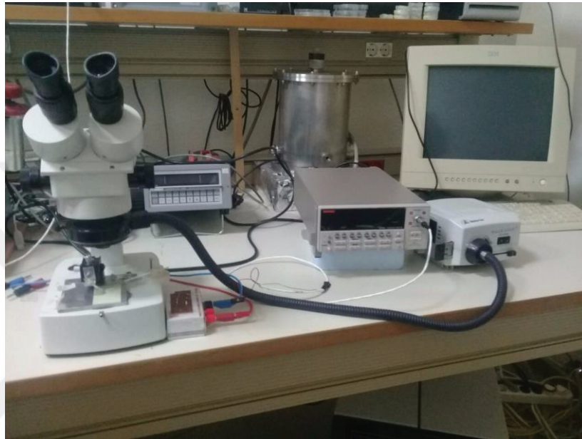
Figure 4.12. I-V experimental setup interfaced with a computer.
