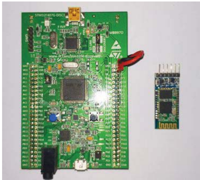
Figure 4.3. STM32F4 Discovery Development Board and HC-05 Bluetooth module
