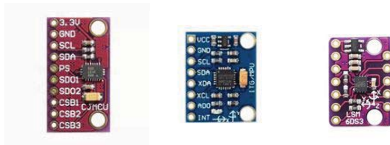
Figure 5.1. MEMS Inertial Measurement Units
