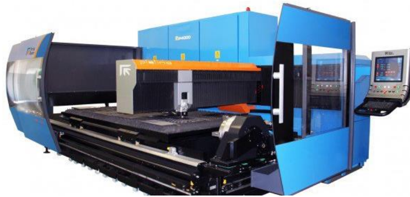
Figure 3.6. Prima Power Platino laser cutting machine with flying optic head.
