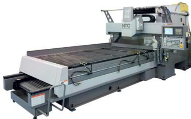
Figure 3.7. Ntclaser TLV Series X-axis moving table and Y-axis moving optics.
