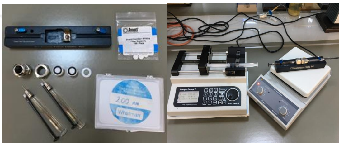
Figure 3.6. Mini-Extrusion parts, Filter supports and Polycarbonate membrane, Hamilton syringes and Pump (Avanti)
