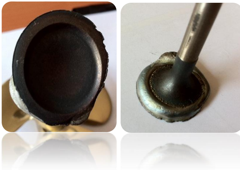
Figure 12.23: Welded Valves with Surface Broken Plat
