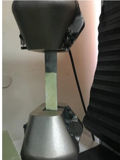
Figure 3.10. Single lap shear test specimen during test
