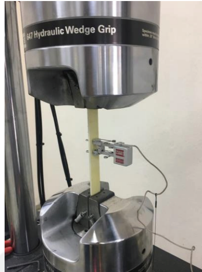
Figure 3.3. Tensile test specimen during test
