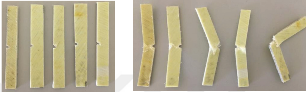
Figure 4.3. Charpy impact test samples (a) before testing, (b) after testing
