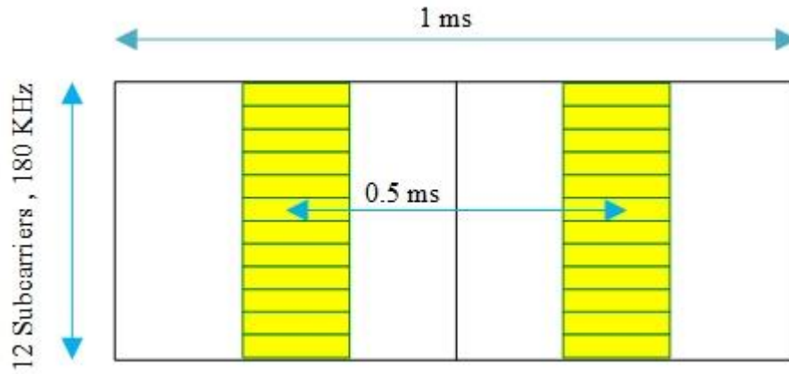
Figure 4.8: 15 K Hz, Resource block configuration (LTE UL, PUSH)
