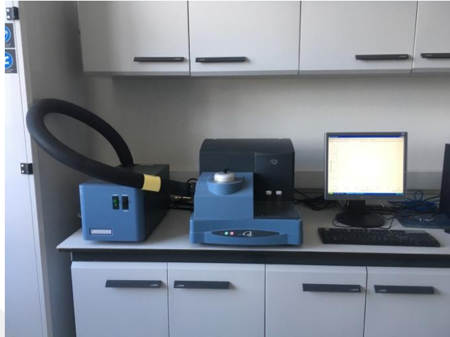
Figure 4.9. TA Instruments DSC Q10 while measuring the specific heat of the tuff sample
