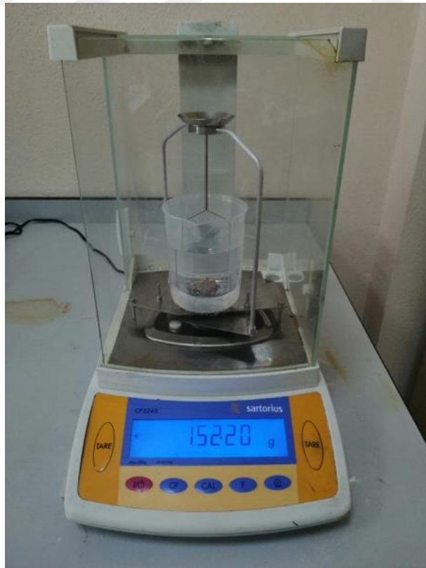
Figure 4.13. The weight of the tuff sample under the buoyancy
