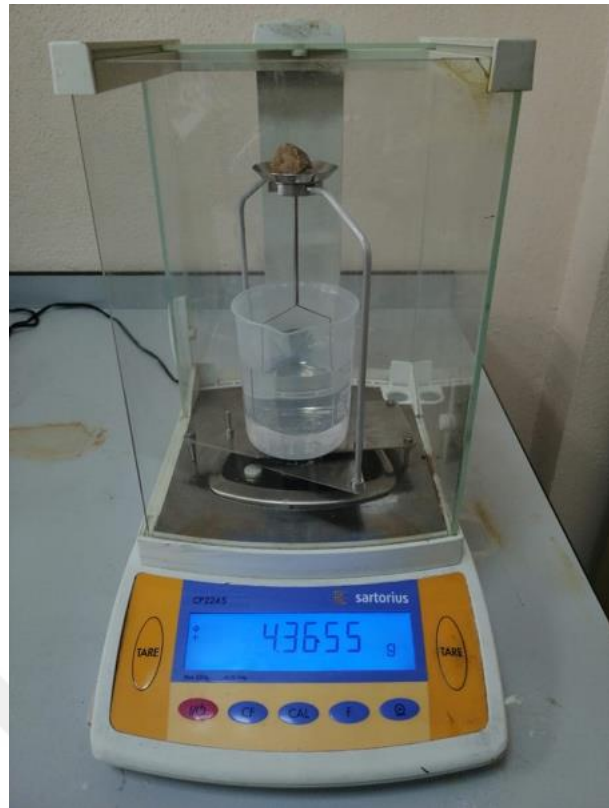
Figure 4.14. The weight of the soaked tuff sample.
