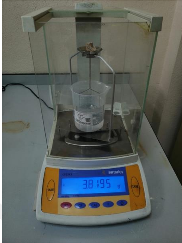
Figure 4.12. The weight of the tuff sample
