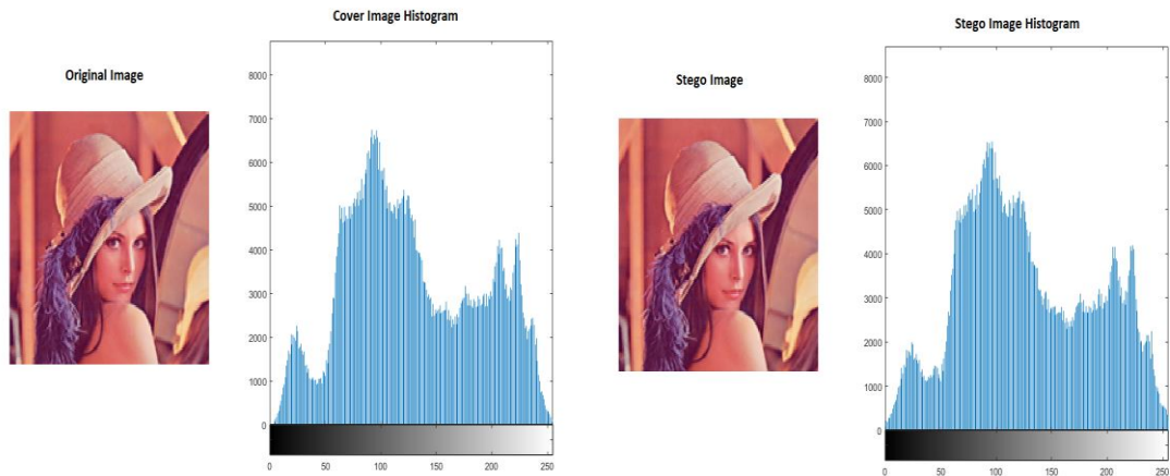
Figure 6.7 Qualitative Comparison for Lena Color Original Image vs. Stego Image with Dimensions (512x512) and their Histograms
