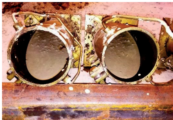
Figure 3.45 Slant Shear specimens
