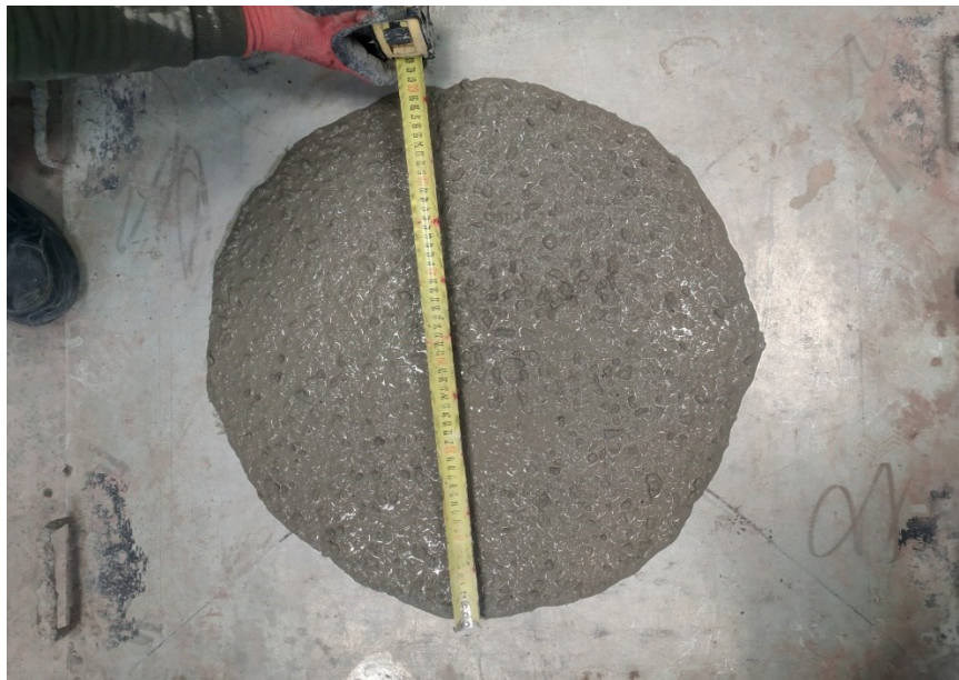
Figure 3.3 Slump Flow Test
