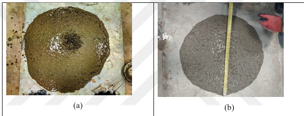
Figure 3.4 VSI = 2 for the left SCC and VSI = 0 for the right SCC
