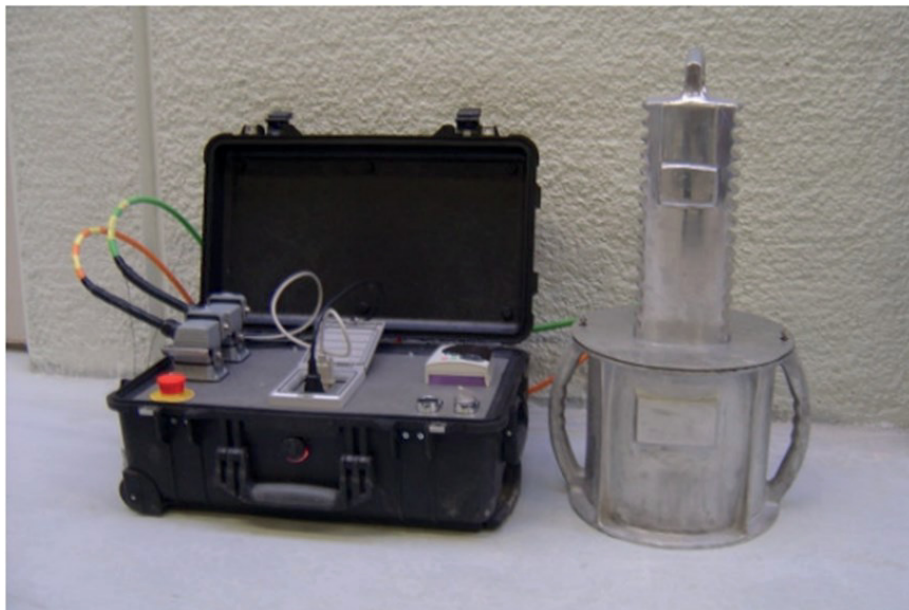
Figure 3.7 Contec 4SCC rheometer
