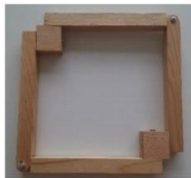
Figure 1.9. Model of a modified Altmann linkage (Source: Atarer, Korkmaz, and Kiper 2017)
