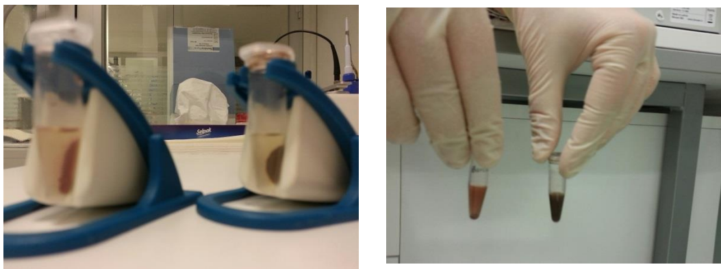
Figure 3.4: Photographs show the magnetic nanoparticles in microcentrifuge tube before and after placed on magnet.
