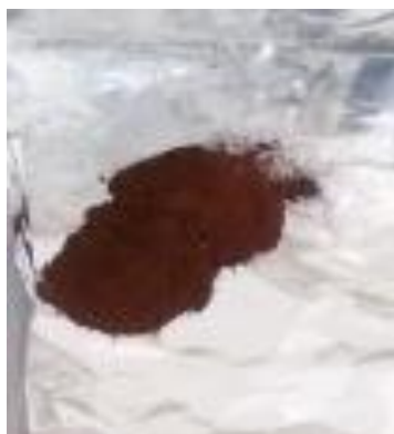
Figure 3.3 : Photograph shows the Fe 2 O 3 nanoparticles after calcination process.
