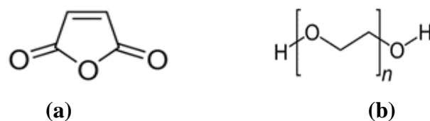
Figure 3.5 : Chemical formula of: (a) MAH. (b) PEG [29].
