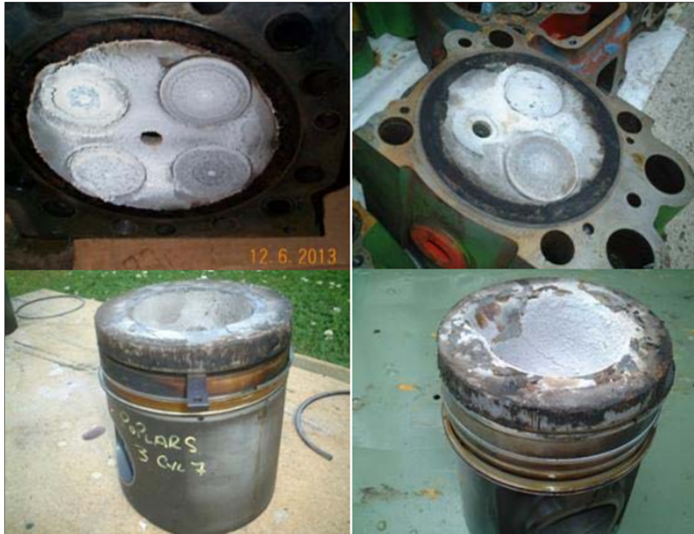
Figure 2.5 : Silica build-up on heads and scrapped pistons of different branded engines.
