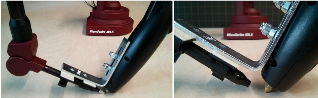
Figure 4.10 : The hybrid tool which integrates the 3D printing pen and the digitizer arm.
