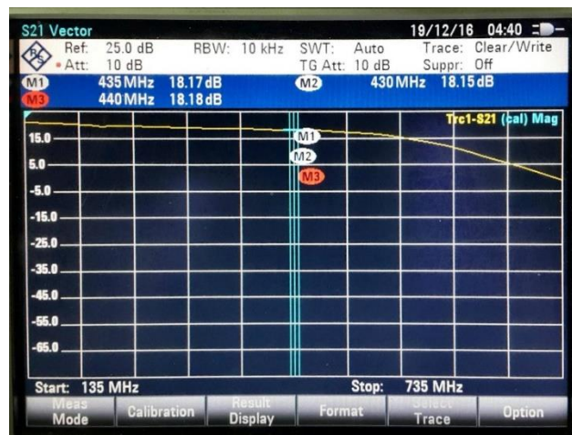
Figure 2. 78: Measurement S21 for Class-E circuit.
