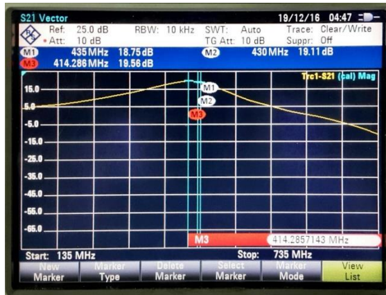
Figure 2. 84: Measurement S21 for Mixed circuit- 56nH.
