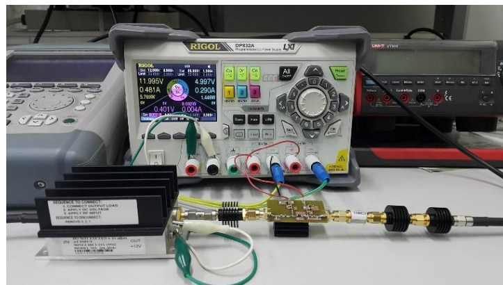
Figure 2. 85: Measurement setup to measure output power.
