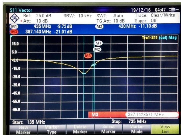
Figure 2. 83: Measurement S11 for Mixed circuit- 56nH.
