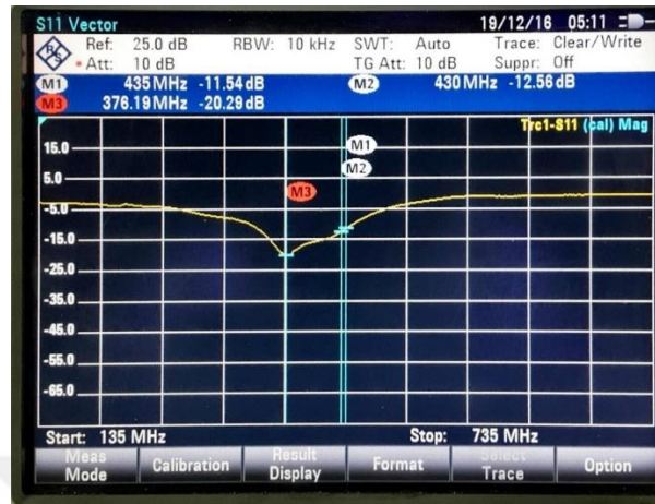
Figure 2. 81: Measurement S11 for Mixed circuit- 47nH.
