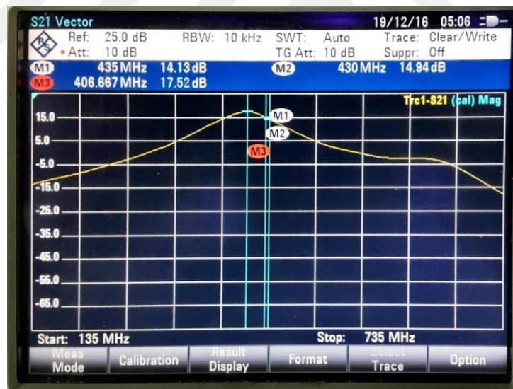
Figure 2. 80: Measurement S21 for Inverse-Class-E circuit.
