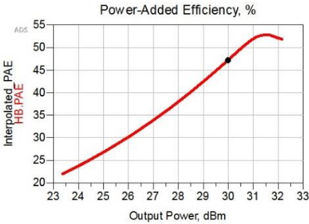
Figure 2. 43: PAE versus output power for Inverse-Class-E design.
