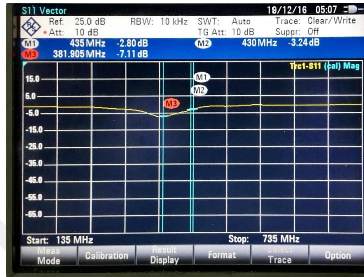
Figure 2. 79: Measurement S11 for Inverse-Class-E circuit.
