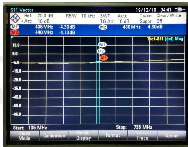
Figure 2. 77: Measurement S11 for Class-E circuit.
