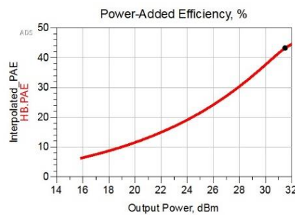
Figure 2. 66: PAE versus output power for Mixed design.
