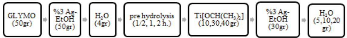
Figure 3. 2 : The recipe of coating solution
