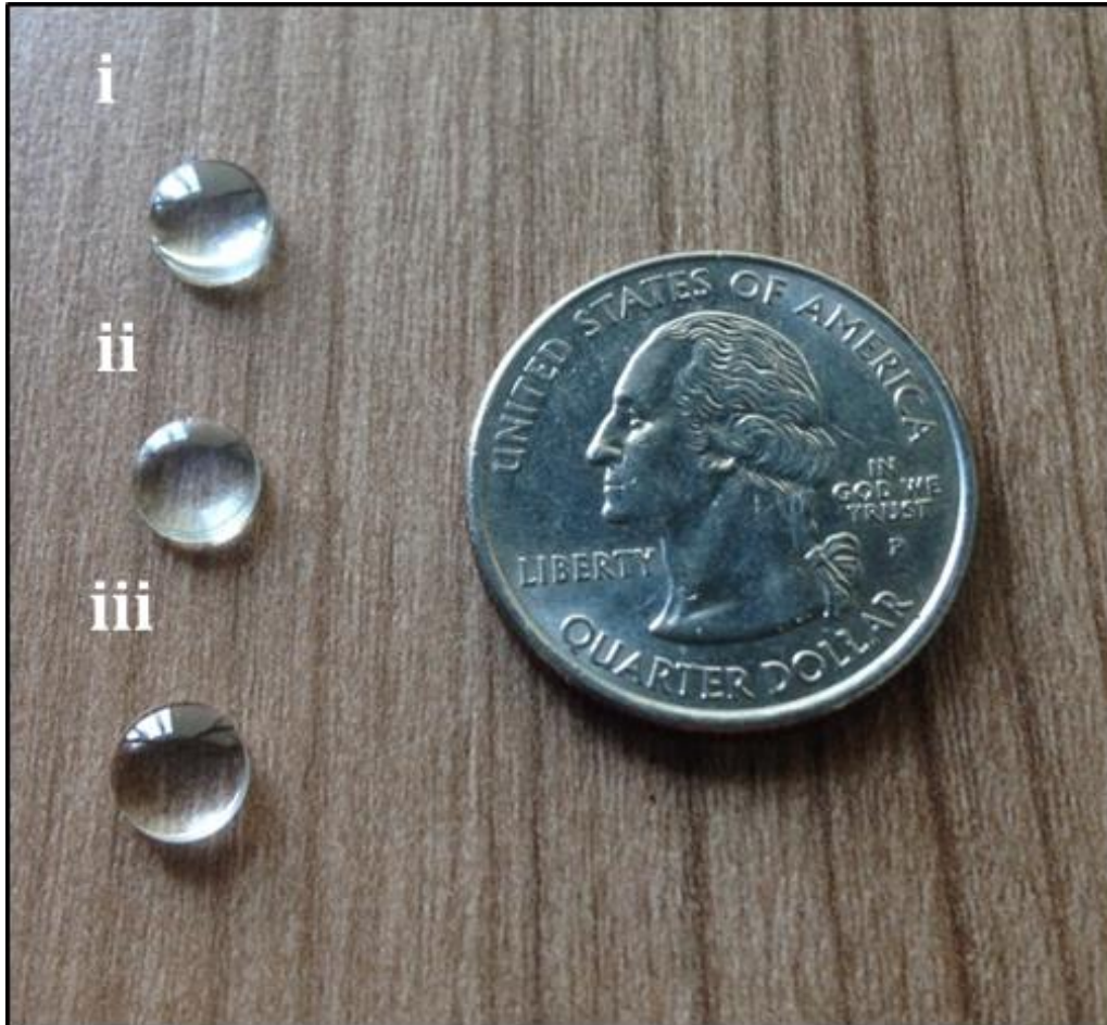
Figure 2.8. i. Commercial 3D Printed Lens, ii.3D Printed Lens (This Work), iii.Commercial Glass Lens.
