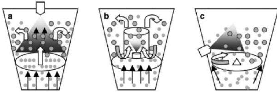
Figure 2.7: Types of a fluid-bed coater. (a) Top spray, (b) bottom spray, (c) tangential spray.
