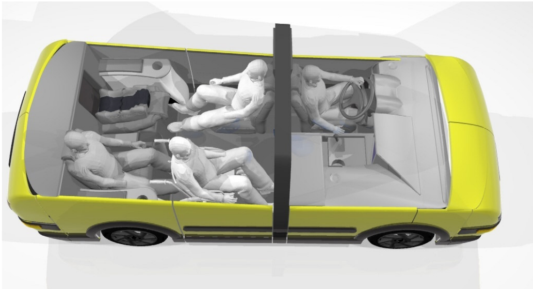
Figure 82: Seating Positions of Four Passengers One of them is Child and One of Them is Disabled
