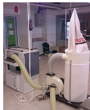
Figure 10: (From left to right) Connection of a machine to the central a central dust collection system (Photography by Alex Velasco taken in Politecnico Di Milano) and a LEV connected to a thicknesser (photography by the author from the model making facility in IEU FFAD)
