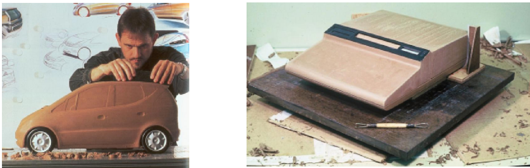
Figure 8: Hard styling clay and examples of its applications in industrial design. Pictures are acquired from Sparke, 2003 (on the left); the webpage www.hp9825.com/html/industrial_design.html (on the right. Accessed in 15 March 2009)
