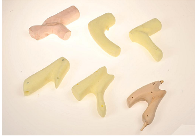
Figure 2: The development of a design through model making- Power hand tool project by Ça da Dorak in the context of the course ID201 instructed by Alex Velasco, 2008 (photography by Alex Velasco)
