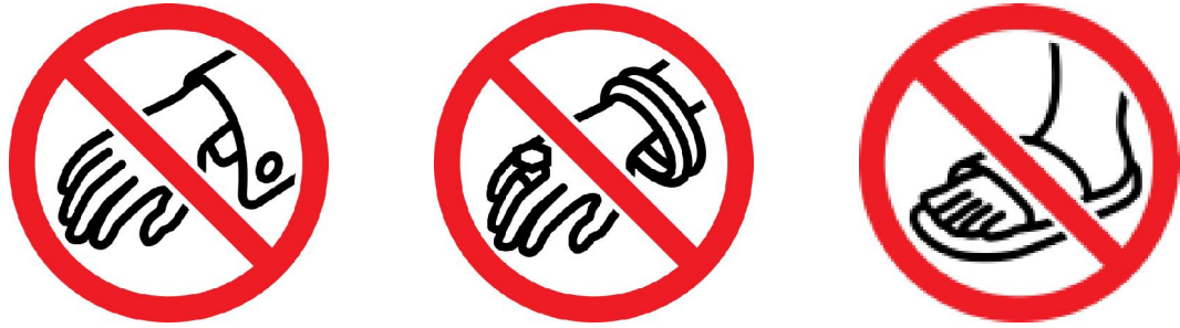
Figure 50: Examples of unique warning signs designed and used by the model making committee in IUE FFAD (designs and illustration by Alex Velasco, 2008). From left to right: “No Loose Clothing”, “No Jewelry” and “No Sandals or Open Shoes”
