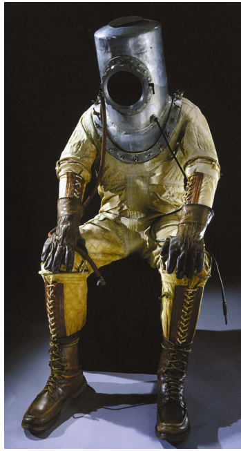
Figure 2.14 Full pressure suit by B.F. Goodrich, USA 1934 (Lee 2005, p.162)
