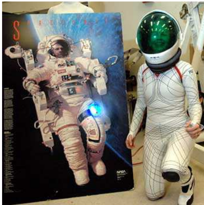
Figure 2.18 Biosuit compared with gas pressurized space suit (Source: MIT Biosuit Webpage, 2009)
