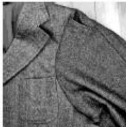
6. make seam straight at front, let a part of the pocket still be seen.
