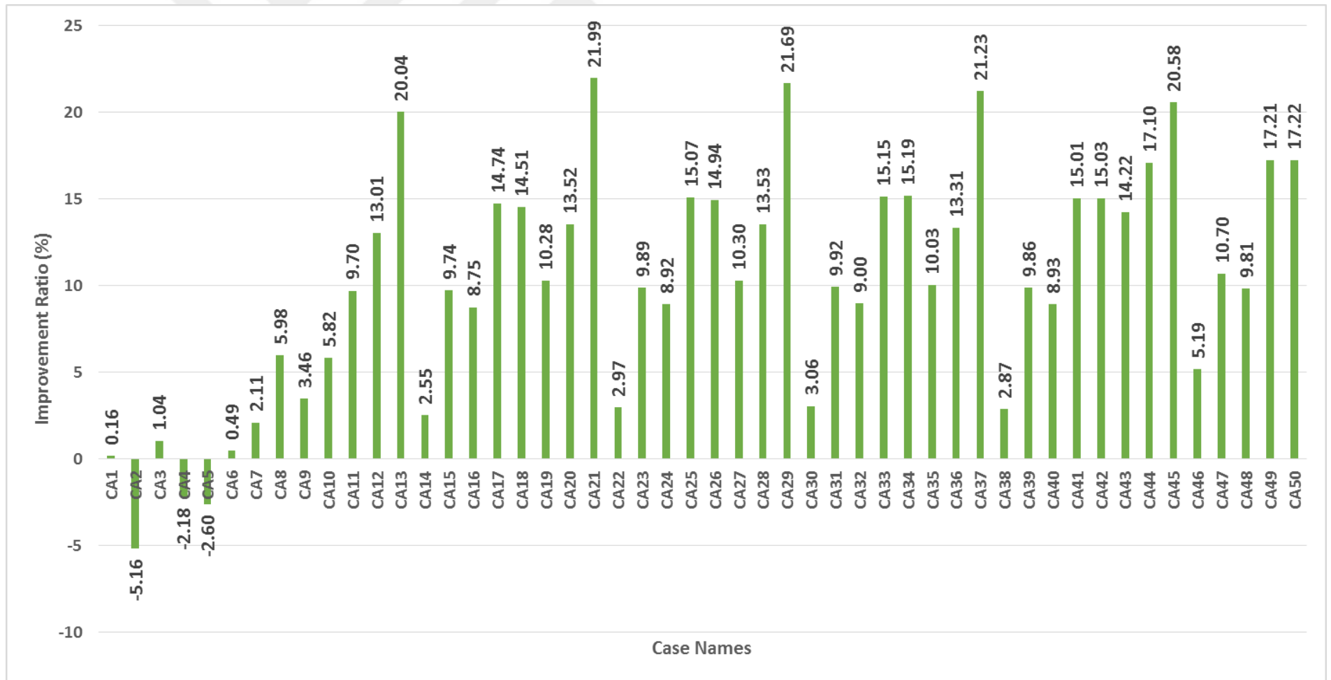
Figure 4.16 : Yearly primary energy performance improvement ratio of the cases in comparison to CA0.
