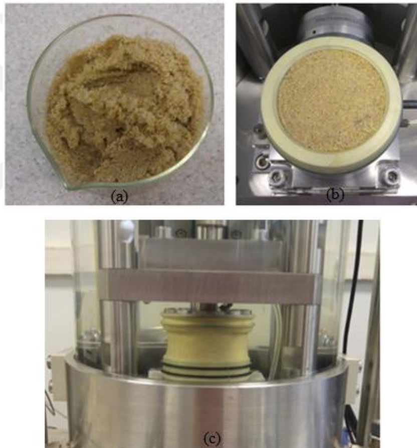
Figure 3.6 : (a)Mixing predetermined amount of water and dry sand in a bowl. (b)Placing the sample into the mold in compacted layers. (c)Specimen prepared by using moist undercompaction method.
