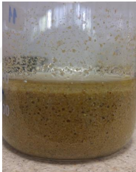
Figure 3.11 : Wet pluviation of dry sand into the mixture of predetermined amount of water and chemical powder.
