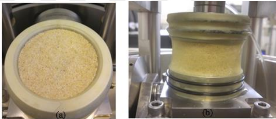
Figure 3.4 : (a)Dry pluviation of sand into the mold. (b)Specimen prepared by using dry pluviation method.
