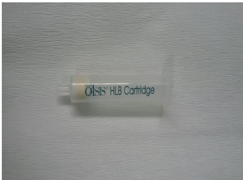
Figure 3.4 : Oasis HLB 6 cc vac cartridge with 200 mg sorbent per cartridge.
