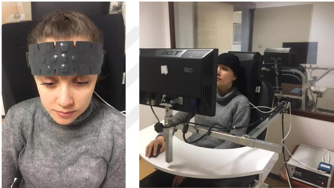
*Figure 8.* Experimental Setup for Study 2. fNIR 200A Model 1200 (left) and experimental equipment in test chamber (right)
