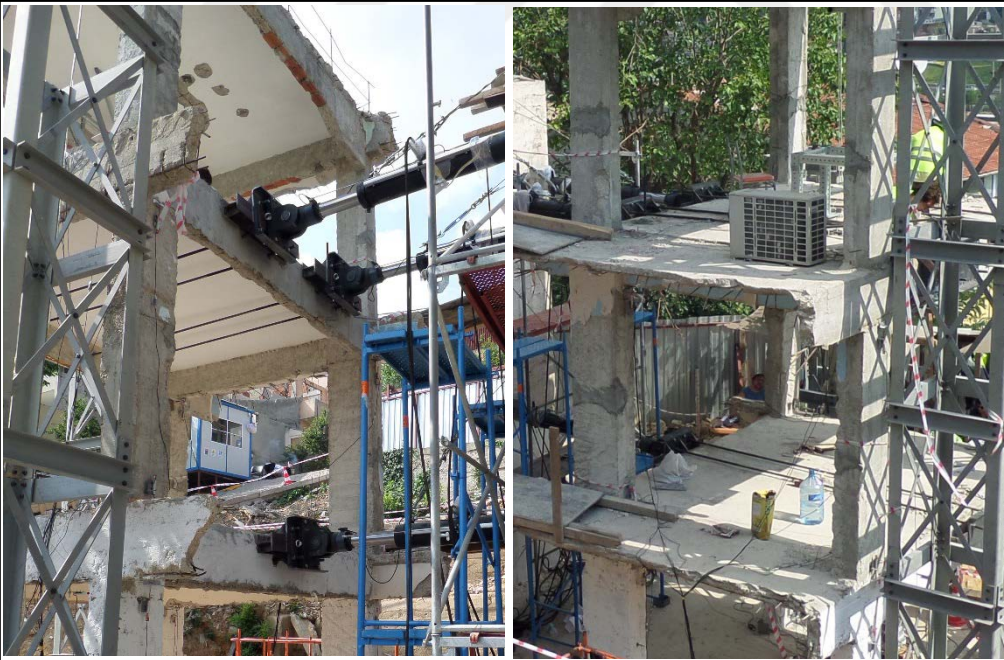
Figure 2.9 : Attachment of the actuators.
