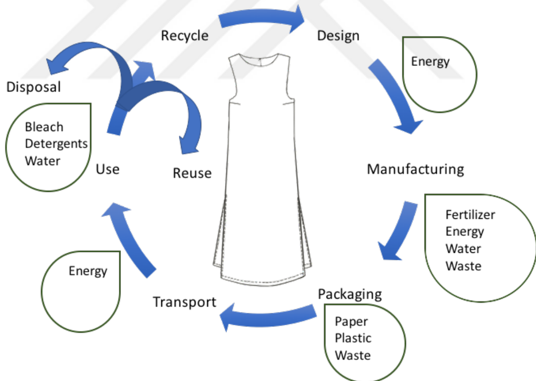
Figure 20 Life cycle assessment of a dress (this model adopted from Koster's (2017) LCA of a t-shirt)
