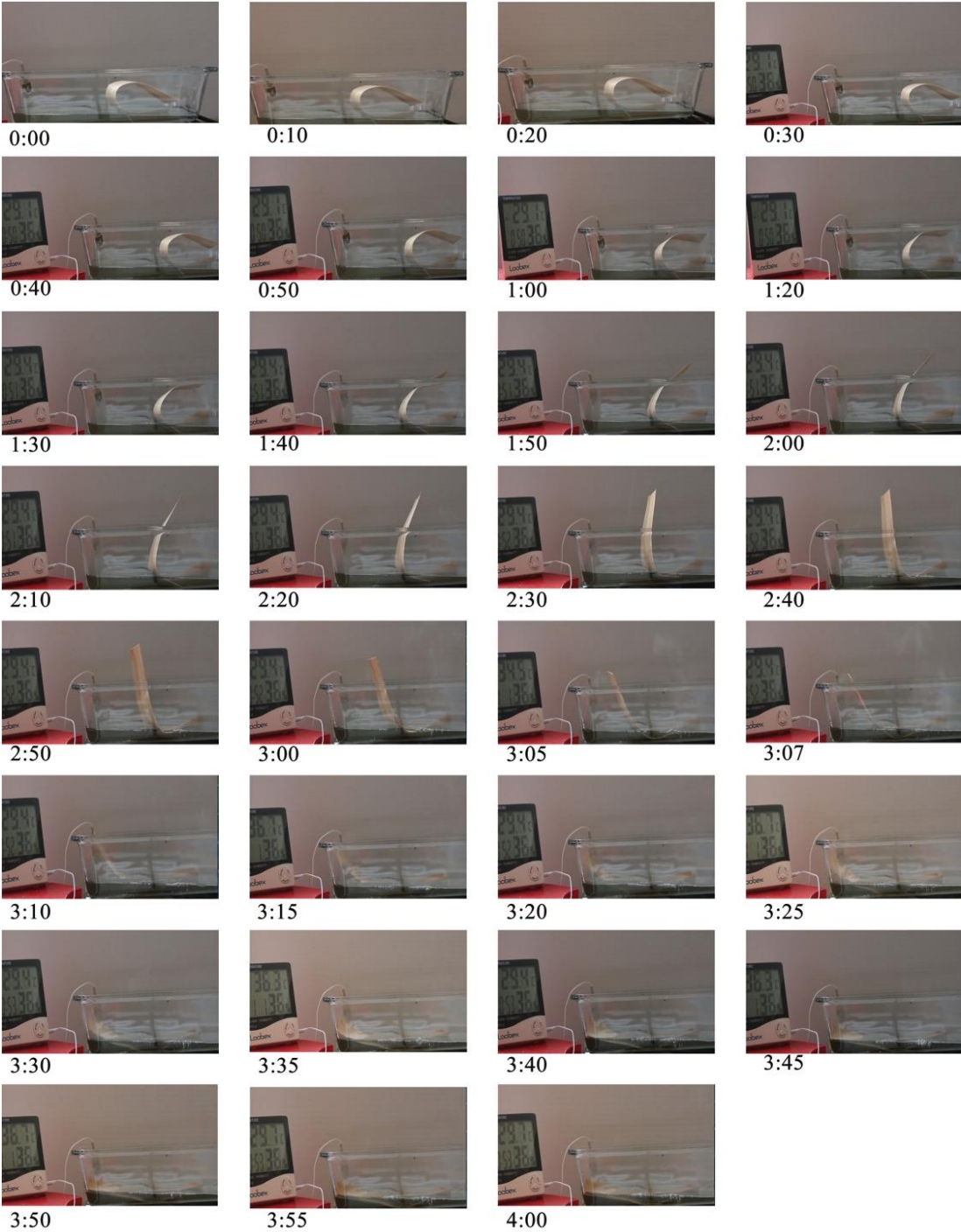
Figure A.1: Experiment to test shape transformation process of oak veneer sample.
