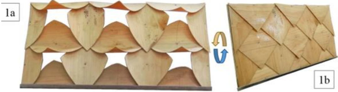
Figure 3.16: Humidity responsive system prototypes by using hygromorphic composites (Holstov et. al, 2015).
