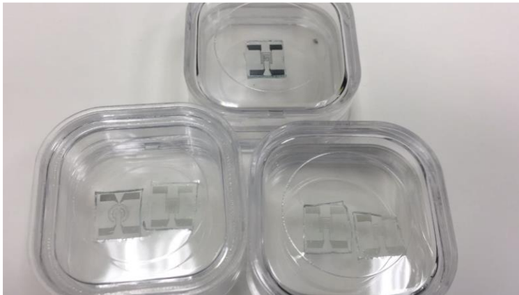
Figure 3.9. The fabricated heating elements
