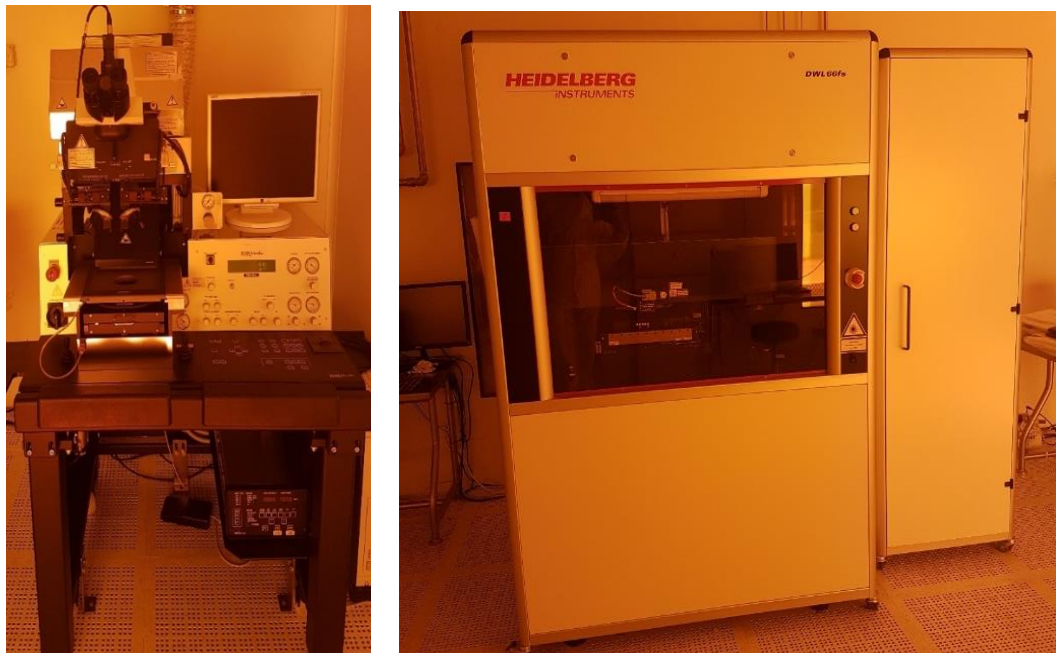
Figure 3.1. a. SUSS MA10 Mask Aligner b The Heidelberg DWL 66fs mask writer.
