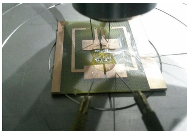
Figure 4.5 Test setup on probe station for measurement of the resistivity of microheater and temperature sensor
