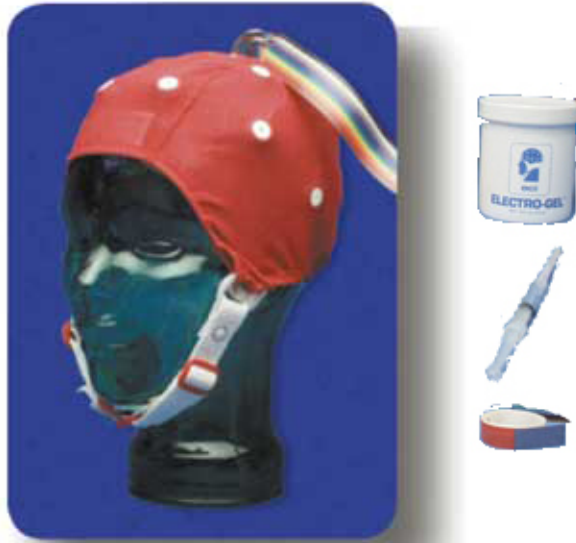
Figure A.2: Bionomadix 10/20 EEG cap is for transferring the patient's live EEG data with wireless communication [31].
