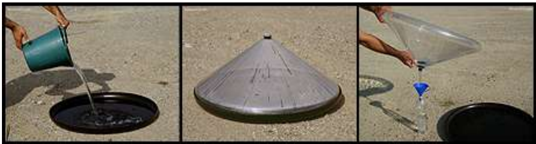
Figure 18 - Desalination with a Water Cone (Watercone, 2018)
