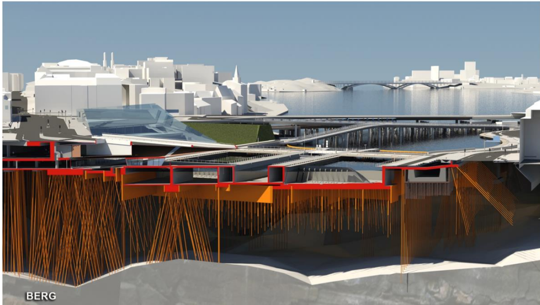
Figure 3.4: model slussen showing 3600 stell piles to be installed.
