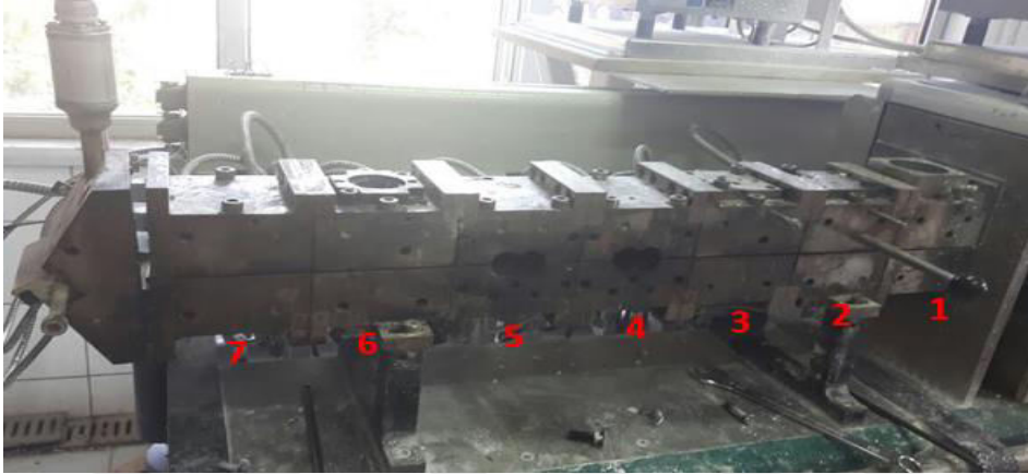
Figure 3.6 : Twin screw extruder and its barrel zones.
