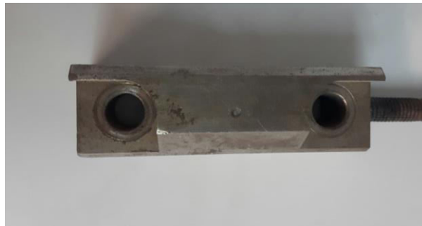
Figure 3.7 : The filamentary die that was used in thesis studies.
