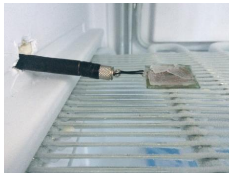
Figure 5.5 : 1[mm] ice covering to surface of the sensor.
