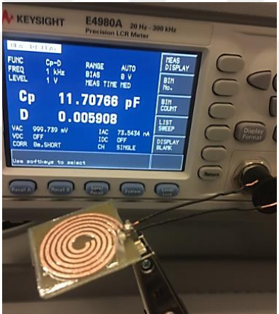
Figure 2.22 : Insulation of the sensor surface via tape at 23°C ambient temperature 50% relative humidity (11,70 pF).
