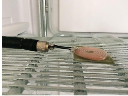
Figure 5.11 : Water drip to all of the sensor surface.
