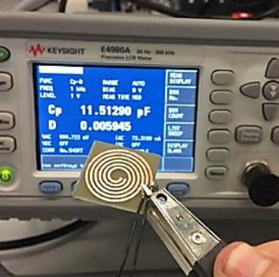
Figure 2.21 : Implemented sensor measurement via LCR Meter at 23°C ambient temperature 50% relative humidity (11,51 pF).
