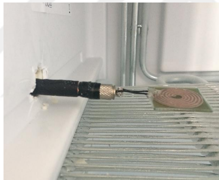
Figure 5.1 : Sensor test without icing in the appliance.
