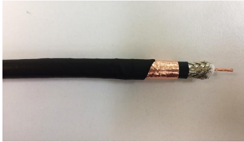
Figure 4.6 : Shielded coaxial cable design (inner one is electrode1, middle one is electrode2, outer one is shield).
