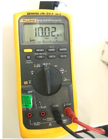
Figure 7.2 : Resistor value 10,02[MΩ] which used in circuit at 25°C temperature.
