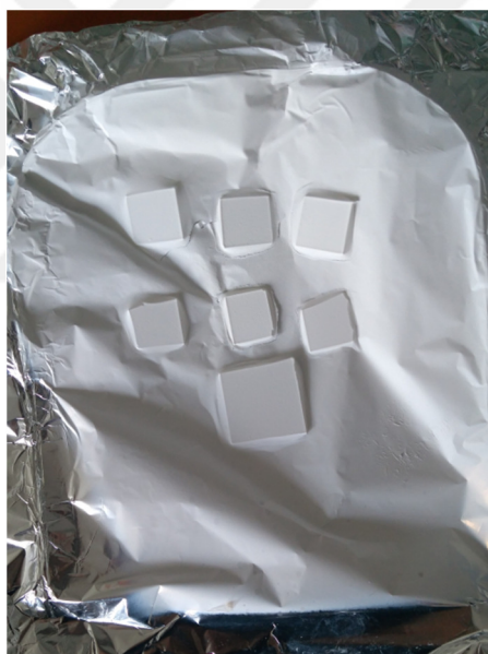
Figure 3.2 : Fiber webs of TB solution electrospun on aluminum foil and glasses.
