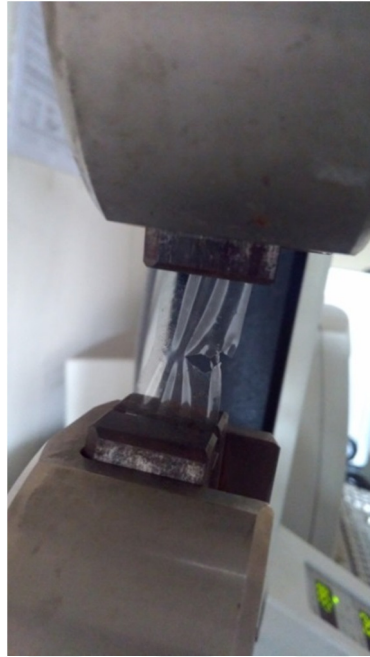
Figure 3.14 : The torn film on the mechanical stress process.
