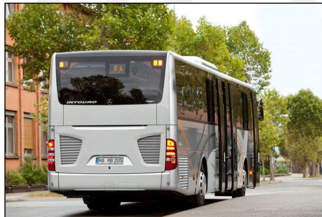
Figure 1.1 : Example of a rear middle bumper integrated to a raised floor bus.
