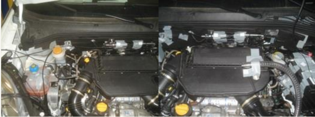
Figure 2.11 : Application of engine ASQ, (Left: operational, 2 microphones for each engine face. Right: Positioning of volume source, at least 2 places on each engine face).
