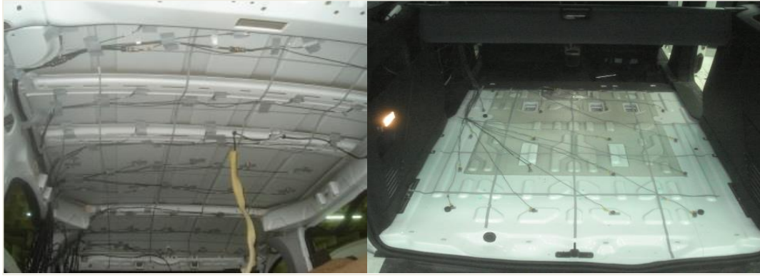
Figure 2.14 : Application of panel contribution (accelerometers on each subpanel), roof (left) and trunk floor (right).
