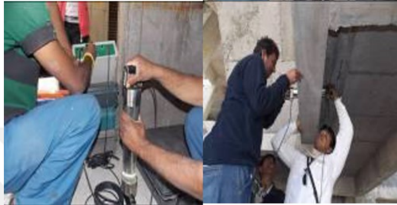
Figure 1. 6: Calibration and UPV test (Kumvat et al. 2014).
