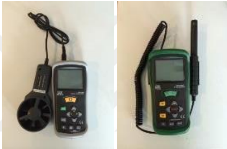
Figure 3.15: Thermo-Anemometer and Humidity meter.
