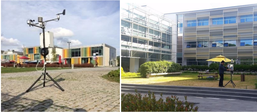
Figure 3.14: Portable mini-weather station during the field measurements.
