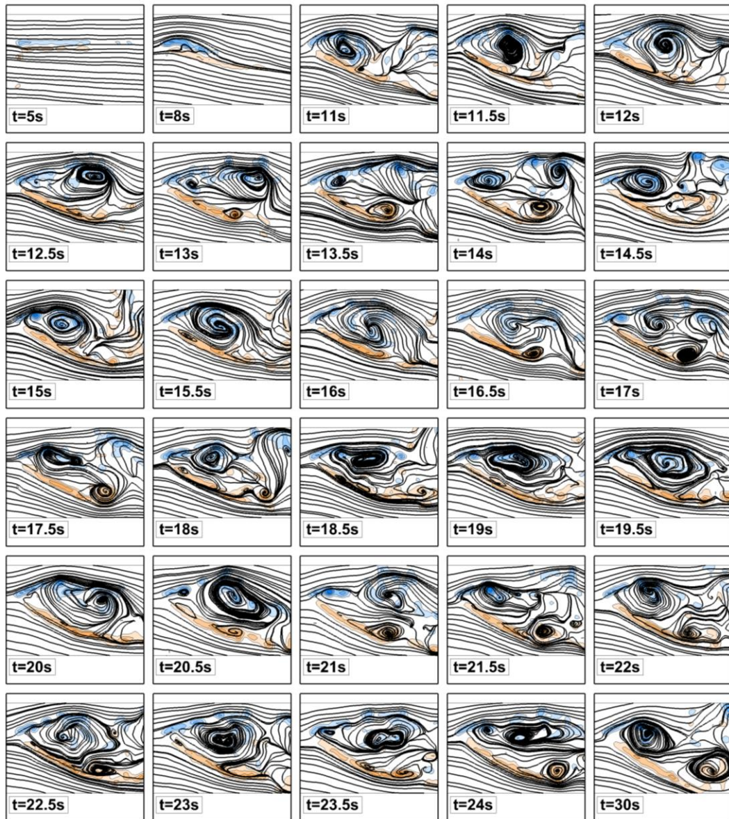
Figure 3.29 : Vorticity contours and streamlines for acetate wing in slow pitch-up motion.
