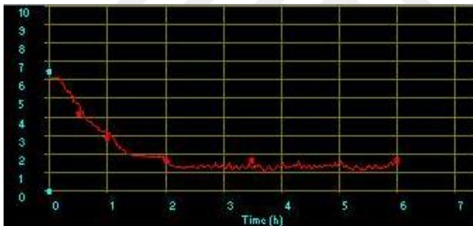
Figure 2.2 : Course of pH in the gastric compartment during the experiments (derived from personal experiments on TIM-1).
