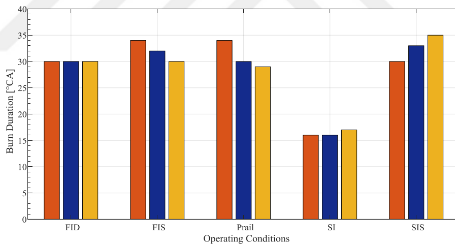
Figure 5.22 : Burn duration comparison at 10 bar IMEP g .
