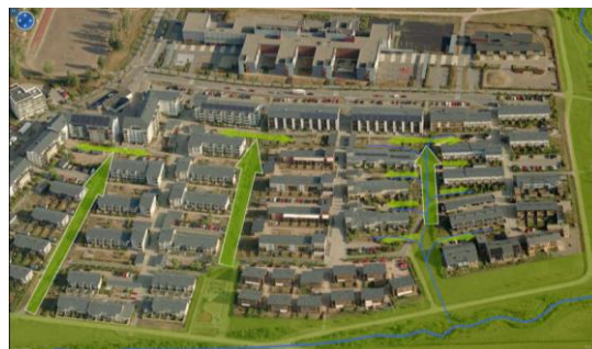
Figure 3.10 : Green Fingers and surface water run-off system in Eko-Viikki (Heikki, 2009).
