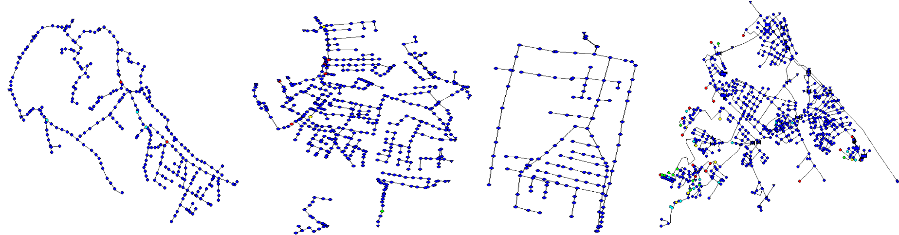
Figure A3.7. Flooded nodes of respectively Uskudar, Kadikoy, Umraniye and Lockwitz regions with their 1-Hour resolution data converted from 1-Minute resolution data
